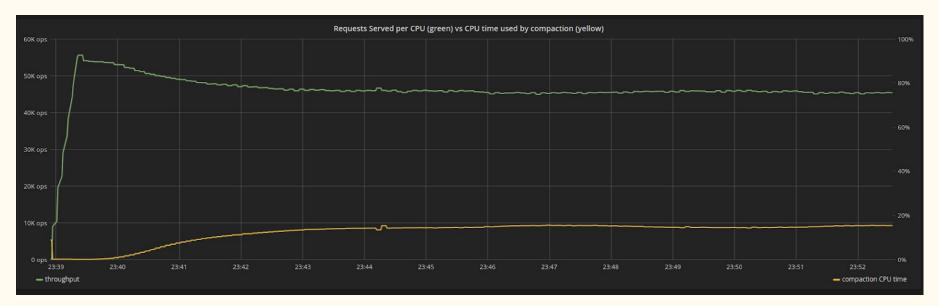
How the system responds to an ingestion-only workload; writing 1kB values into a fixed number of random keys so that the system eventually reaches steady state.
