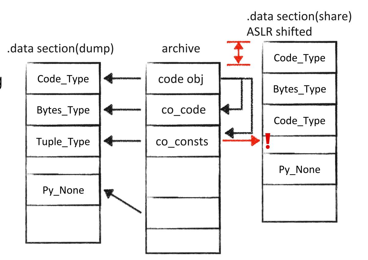
MAP\_FIXED ensures that the pointer inside the archive is correct, but ASLR causes the pointer to the data section invalid. Iterating over the object graph to fix the pointers.
